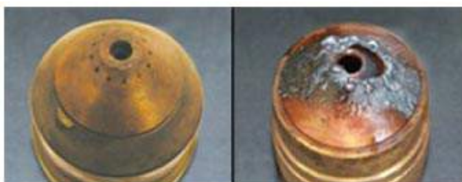
300 pierces at 50 mm (2") HPR400XD with PowerPierce technology
