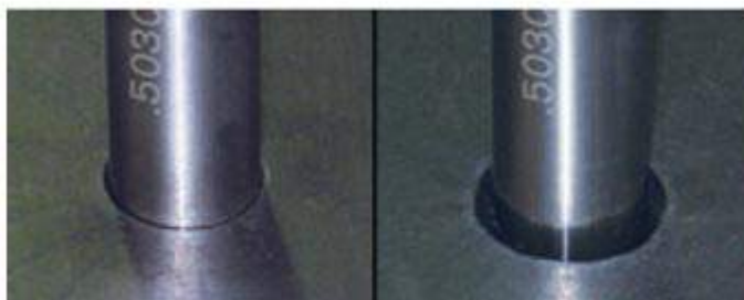
12 mm (1/2") hole with True Hole technology
