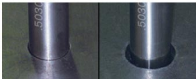
12 mm (1/2") hole with True Hole technology
