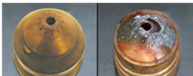
300 pierces at 50 mm (2") HPR400XD with PowerPierce technology
